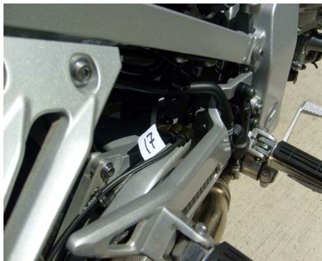
REAR LINE ROUTING DOWN THE SWING ARM
