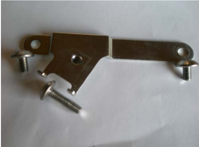
A3 REMOVE O.E.M BRAKE LINE BRACKET
