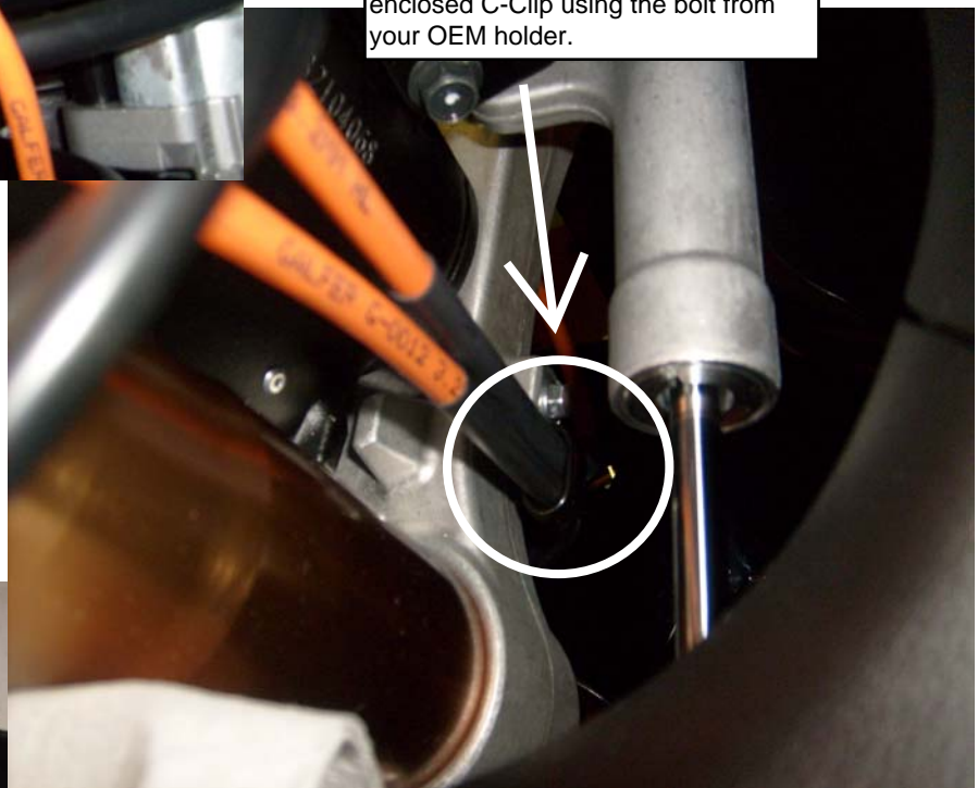
Picture C: OEM Shield Please remove this shield from the lower triple clamp to ease installation of your Galfer brake lines.
