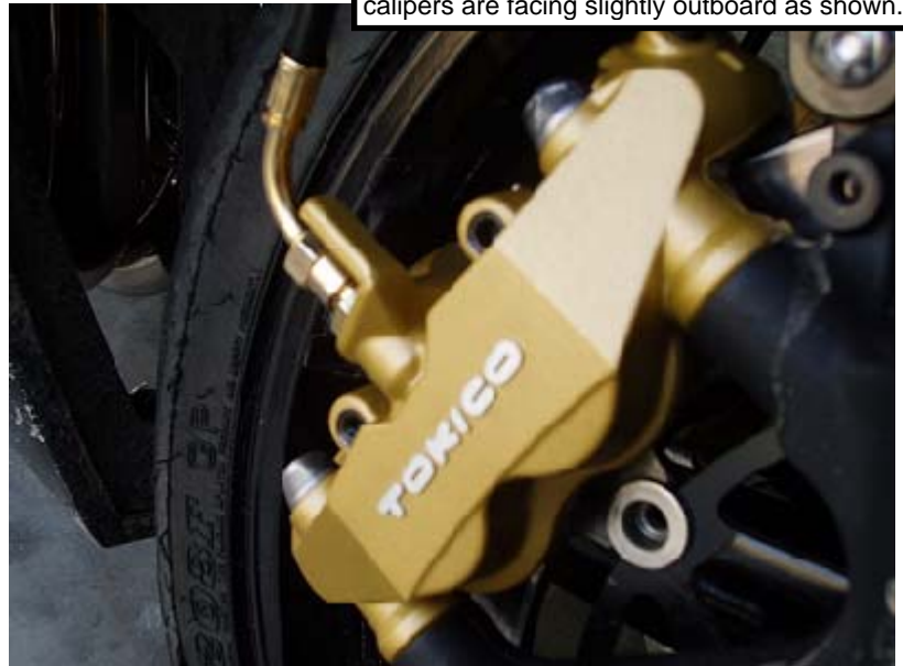
Picture B: Calipers Please make sure the fittings at right and left calipers are facing slightly outboard as shown.
