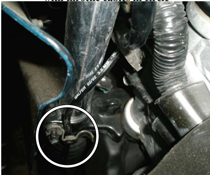
B-1. Line from the control panel to left fork, line routed through OEM clip in circle
