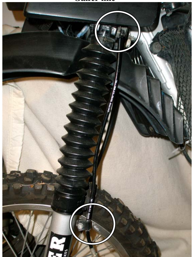
B-2. Left Fork overall, line routed through OEM clips in circles
