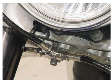
c. Galfer t-block at lower triple tree
