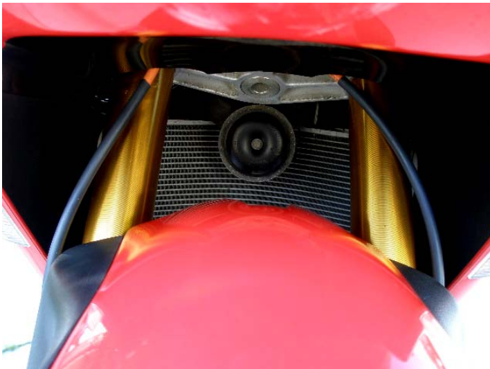
c. Right and left lines routed in front of the forks
