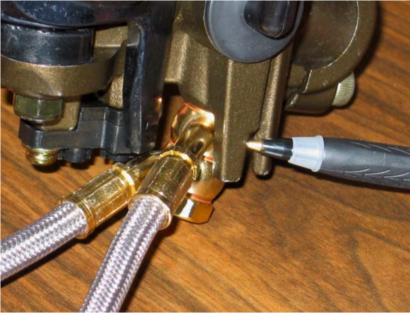
Master Cylinder Modification Example to the right: Galfer lines installed with master cylinder on bike, pen and "X" indicate which tab to grind off
