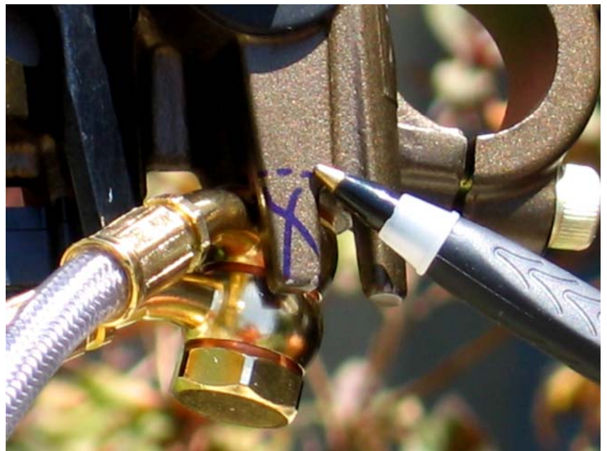
Master Cylinder Modification Example to the right: Galfer lines installed with master cylinder on bike, pen and "X" indicate which tab to grind off
