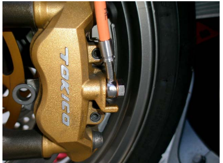
d. Left caliper, notice banjo position
