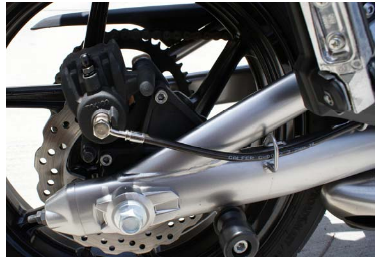
B. Line routed down the swing arm through OEM line holders to the caliper
