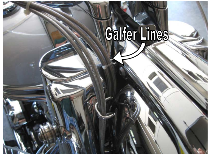
b. Galfer lines routed from the master cylinder
