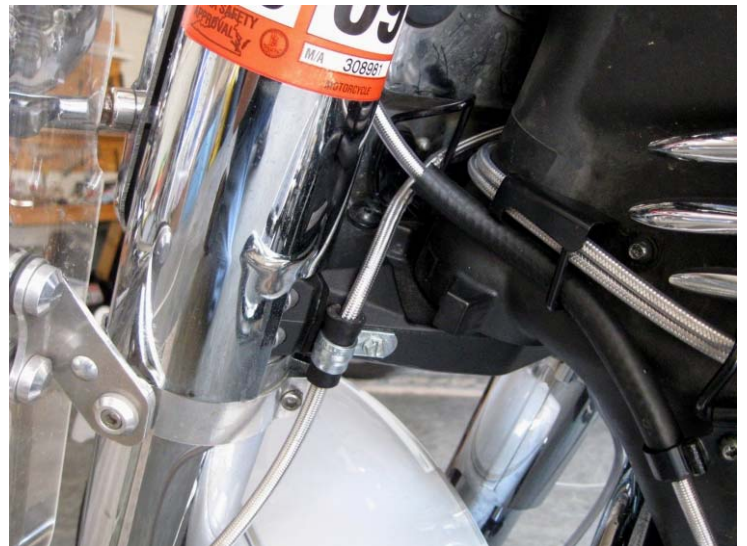
d. Left line routed above the triple tree
