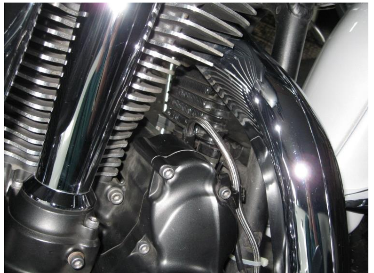
f. Routing at oil cooler
