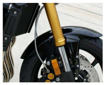
d. Overall routing to calipers
