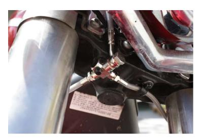
c. Lines A, B & C – T-block and Galfer c-clip at the lower triple tree
