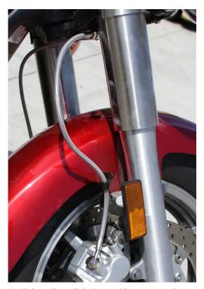
d. Line B – Right caliper routing
