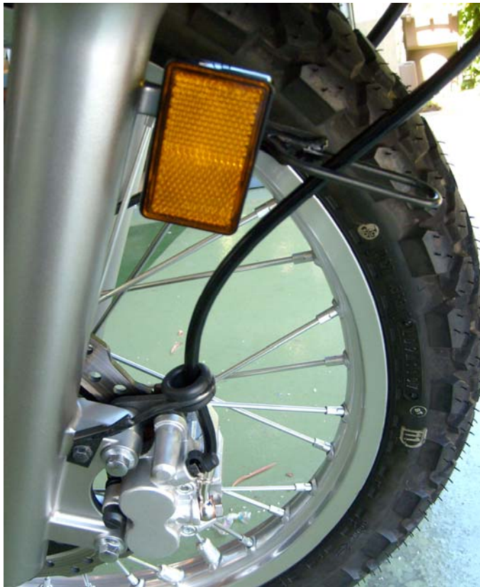
c. Left caliper, Galfer line routed through both OEM line holders
