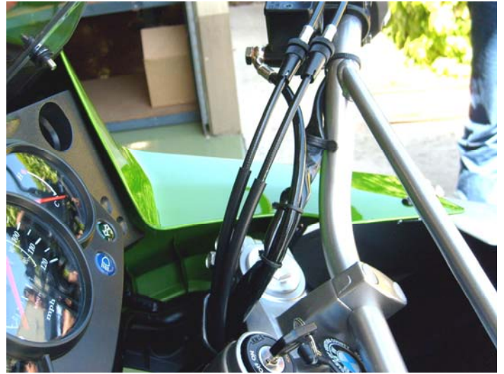
b. Galfer line routed through OEM bracket and zip-tied to the electrical hose
