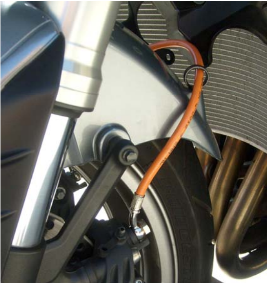
g. LINE C – Left caliper routing
