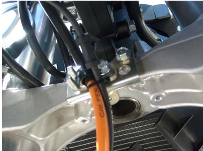
d. LINE B – Galfer c-clip at lower triple tree
