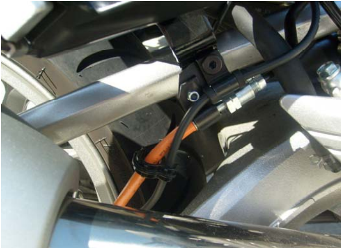
i. REAR LINE – Galfer sheath clamp at OEM hard tubing
