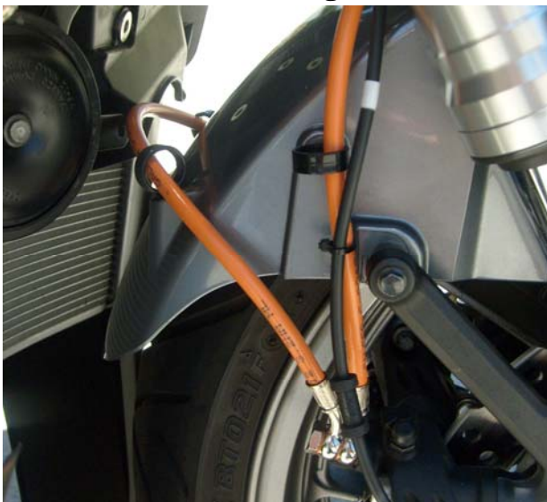
e. LINES B & C – Right caliper, notice OEM routing tabs
