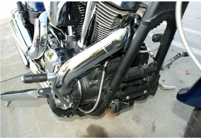
c. Routing at oil tank
