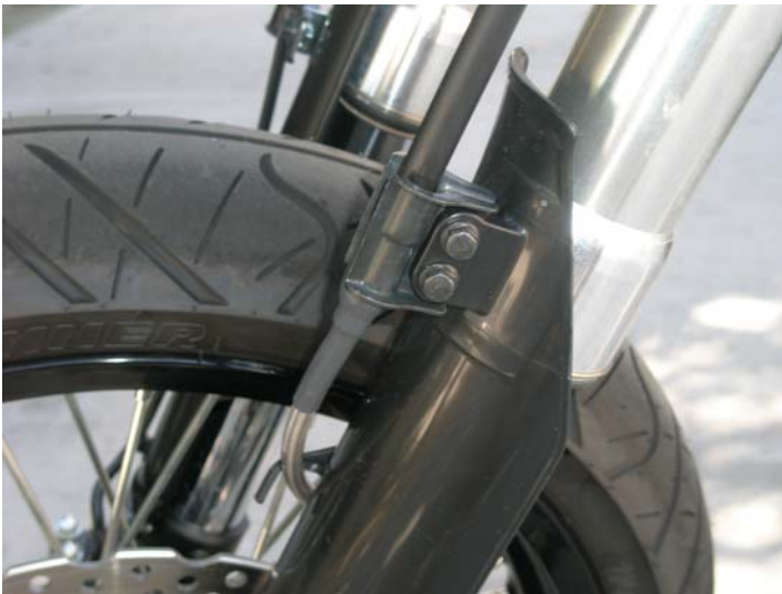
C. Notice the line routing through OEM Line Holder and behind the Fork
