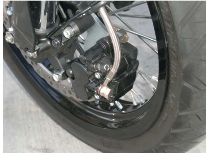
D. Line routing through the Guide Bracket and to the Caliper
