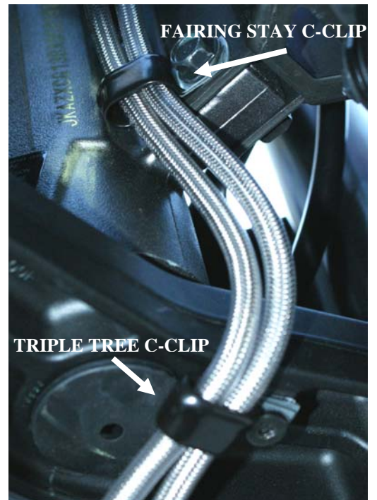
B. C-clip at Fairing Stay and C-clip at Lower Triple Tree
