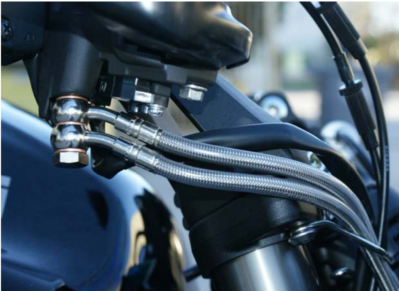
A. Master Cylinder with lines through guide bracket
