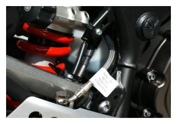
Line H – Rear Master Cylinder, notice Line I routing
