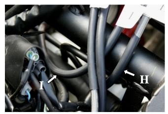
Lines I & H – Routing from ABS Unit towards Swing Arm
