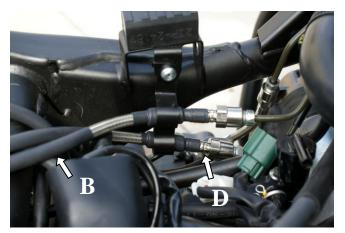
Lines B & D – Routing from ABS Unit to OEM tubing
