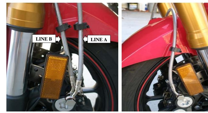
C. Lines A & B at Left Caliper
