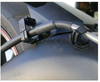
**B.** Rear line through stock guide brackets
