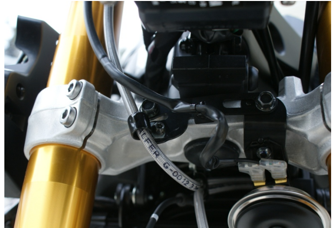
Line-A routing using a Clip-1 @ lower triple
