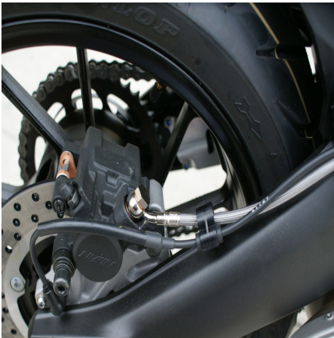
Line -E rear caliper to ABS unit using OEM routing and tabs
