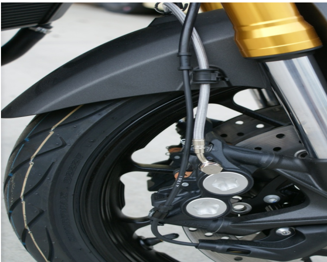
Right caliper Line-B crossover to left
