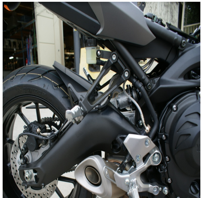
Line-D rear master cylinder to ABS unit
