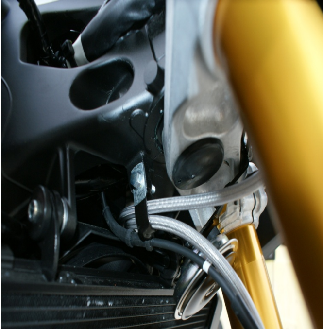
Lines-A/C routing using Clip-2 from front master and left caliper to ABS unit
