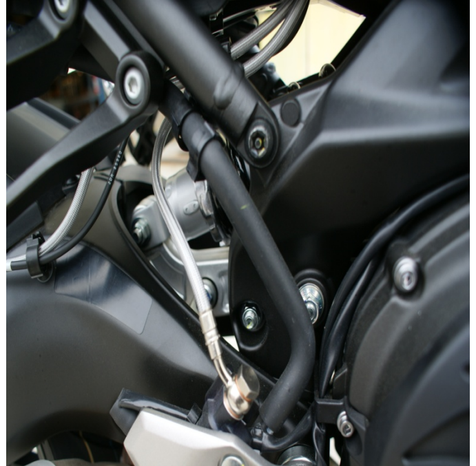
Line-B from A.B.S. block to rear master cylinder
