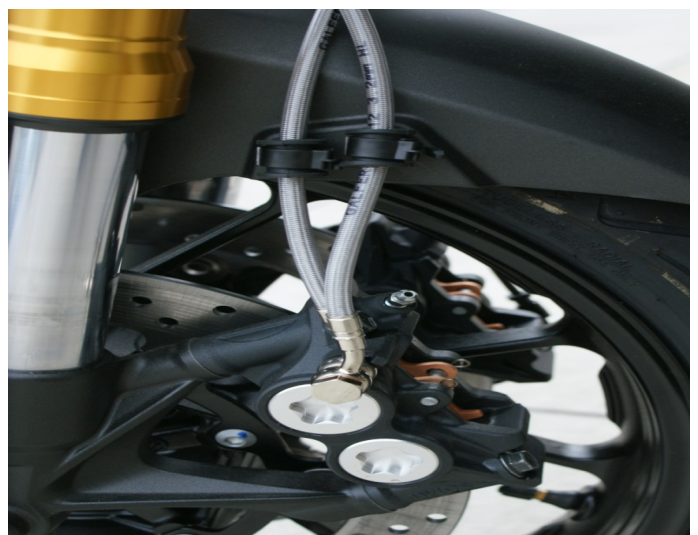
Left caliper Lines-B (inner) crossover from right caliper Line-C from ABS unit
